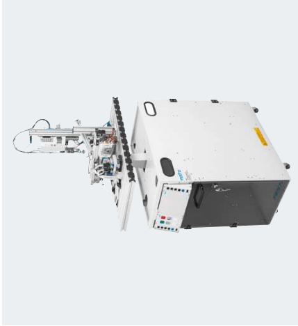
Station Pick&Place with additional equipment
